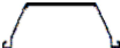
Flat / Straight Type (SA), (S): Used for filled cell construction
