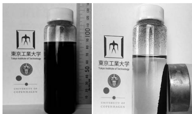
Magnetic Carbon Nanotubes before (left) and after (right) introducing a permanent magnet.
