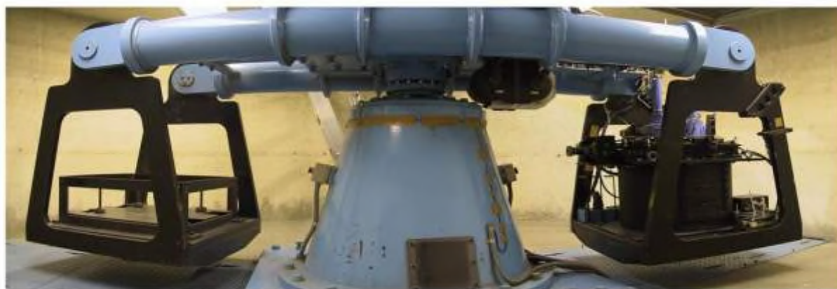
図 1 Tokyo Tech Mark 3 Centrifuge (Since 1997)
